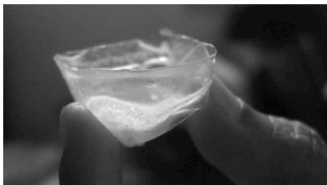
Figure 4 Picture of the second PMMA and \text{EuD}_4\text{TEA} sample taken using natural light. A full color version of this figure is available at Polymer Journal online.
