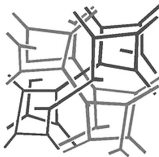
Figure 8 Bicontinuous cubic phase with the space group Ia3d . 26 A full color version of this figure is available at Polymer Journal online.
