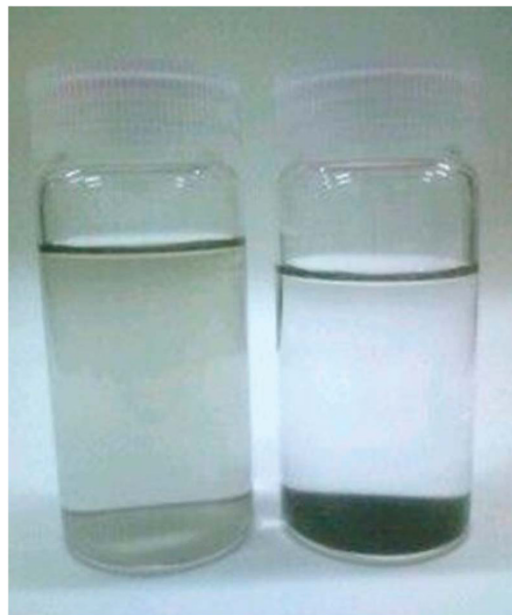
Figure 3 A photograph of LPEI ( M_w 25 000)-protected PtNPs dispersed in water at pH 4 (left) and precipitation at pH 7 (right).
