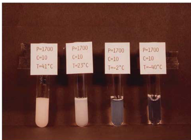
Figure 3 Photographs of poly(vinyl alcohol) gels in mixtures of dimethyl sulfoxide and water (60/40 v/v) at various gelation temperatures T_q s. T_q = 41 , 23 , -2 , -40 °C from left to right.
