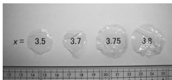
Figure 5. Dried composites after equilibrium at x = 3.5, 3.7, 3.75, and 3.8 .
