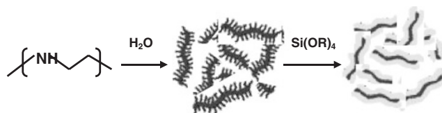
Scheme 1. Schematic representation of LPEI aggregation and silica deposition.
