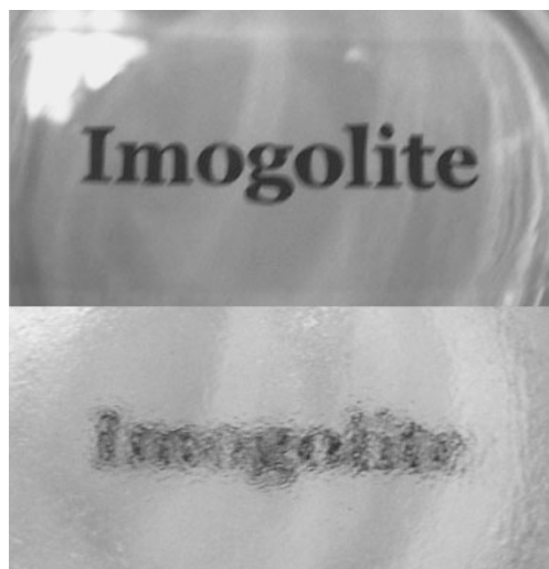
Figure 20. Transparency of in situ hybrid (upper) and blend (lower) films with imogolite:PVA = 1:20. The thickness of films is ca. 100 μm Reprinted with permission from K. Yamamoto, et al. , Soft Matter , 1 , 372 (2005). 47 © 2005, Royal Society of Chemistry.
