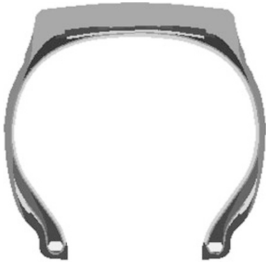
Figure 7. The sectional geometry and material distribution of the truck tire.
