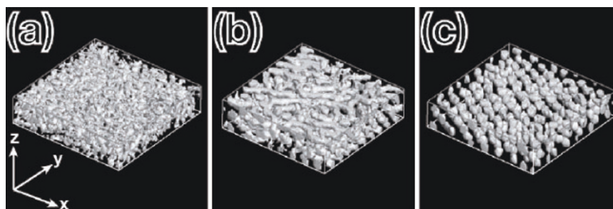
Figure 2. 3D morphologies of Poly(styrene- block -isoprene) (SI) block copolymer thin film. 62 The number-averaged molecular weight and polydispersity index are M_n = 51,000 and M_w/M_n = 1.06 , respectively. The volume fraction of polyisoprene is 0.22. A specimen film was prepared by spin-coating from toluene solutions with 2.6 wt % onto the mica substrate. Microphase-separated structures of (a) as-spun film and annealed at 120 °C for (b) 2880 minutes (48 h), (c) 9000 minutes (150 h) under vacuum. Polyisoprene phase is shown Box size: 300 \times 300 \times 70 nm.
