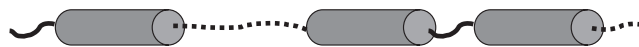
Figure 15. Illustration of main-chain LC polymer with two different spacers sequenced in a regularly alternate fashion.
