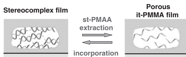
Figure 12. Schematic representation of the selective extraction of st-PMAA from the LbL assembly of it-PMMA and st-PMAA on the basis of stereocomplex formation, and the subsequent incorporation of st-polymers of methacrylic acid or methacrylates. Reprinted with permission from T. Serizawa et al. , Angew. Chem., Int. Ed. , 42 , 1118 (2003). 64 © 2003, Wiley-VCH.
