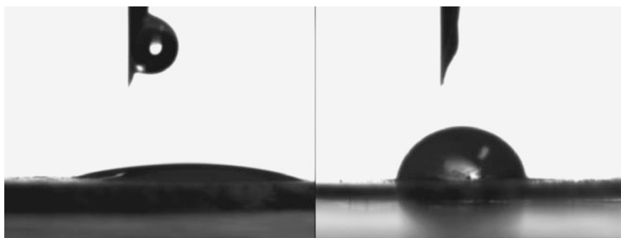
Figure 7. Contact angles of glycerol drops in halloysite (left) and g-halloysite (right) surface.
