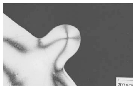
Figure 1. Polarizing optical photomicrograph of Schlieren texture for EDMB-10 quenched from the melt to 0 °C, which was taken under crossed polarizers at 4 °C.
