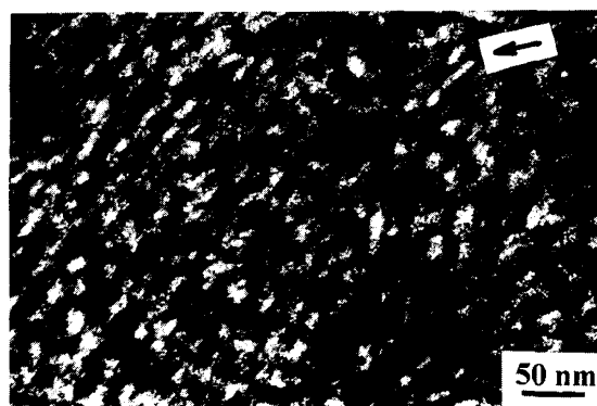
Figure 12. TEM micrograph of PP/hBR (50/50) blend quenched to 0^{\circ}\text{C} and then annealed 17 h at 140^{\circ}\text{C} .
