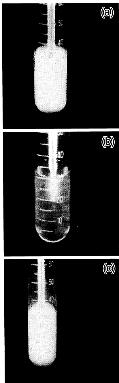
Figure 3. Photographs of o/w emulsion prepared with chitosan aqueous solution, decalin and Nonipol 110 (HLB 13.8, cloud point 70–76°C) at different temperatures: (a) room temperature; (b) 60–70°C; (c) 85°C.
