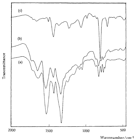
Figure 3. Infrared spectrum of poly(thiophene) (a) obtained from Run 1 in Table I, (b) obtained from Run 15 in Table I, and (c) obtained from Run 16 in Table I.
