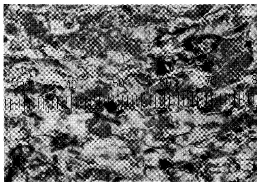
Figure 10. POM photograph of polyamide 3c at 121.5°C on cooling cycle, \times 150 .
