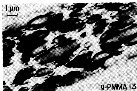
Figure 2. Transmission electron micrographs of AIBN membranes.
