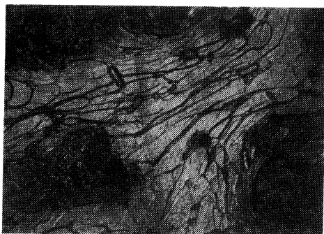
Figure 5. Microphotography for the equimolar mixture of Polymer I and Polymer III taken at 178°C (Magnification 100×).
