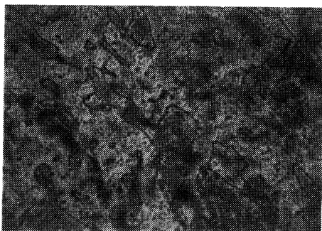
Figure 4. Microphotography for the equimolar mixture of Polymer I and Polymer II taken at 241°C (Magnification 100×).
