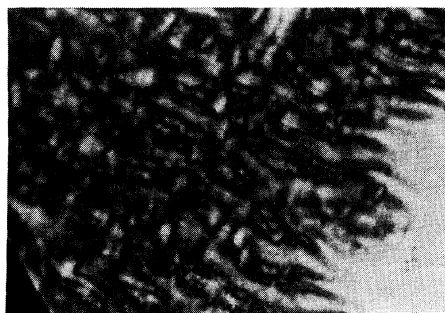
Figure 7. Photomicrograph (original magnification 50X) of Williams domains formed after 30 min in a copolymer of ChMA-BMA (0.83:0.17) at 155°C (40 V dc).
