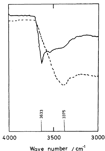
Figure 3. IR-spectra of Aerosil 130 immersed in (—) nitroethane and (---) 4-vinylpyridine monomer.
