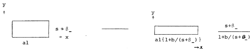
Figure 9. Schematical illustration of the dimension before and after drawing to x -direction.
