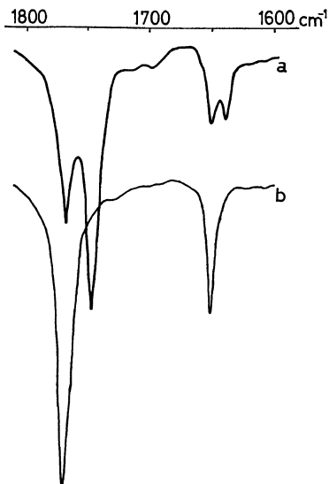
Figure 6. IR spectra comparing VAc—( \text{AlEt}_3\text{—ZnCl}_2 complex) mixture with a reference system: a, VAc— \text{AlEt}_3\text{—ZnCl}_2 (1:1:1, ca. 10 min after preparation); b, free VAc (quite similar to the spectra obtained for the system VAc— \text{AlEt}_3 (1:1), VAc— \text{AlEt}_2\text{Cl} (1:1), or VAc— \text{ZnEtCl} (1:1)); each 0.1 molar solution of THF; 23^\circ\text{C} .
