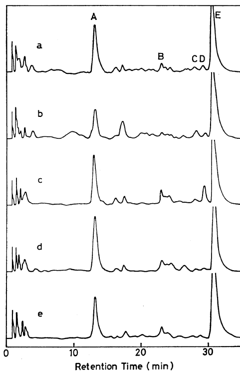
Figure 8. Profiles of CPP—GLC with cello-oligosaccharides: (a) cellobiose; (b) cellotriose; (c) cellotetraose; (d) cellopentaose; (e) cellohexaose.
