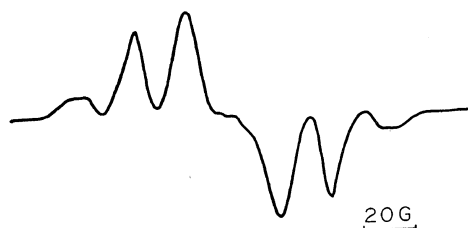
Figure 4. ESR spectrum of isoprene 1 mol% in n -butyl chloride glass matrix measured at 77°K following \gamma -irradiation at 77°K.
