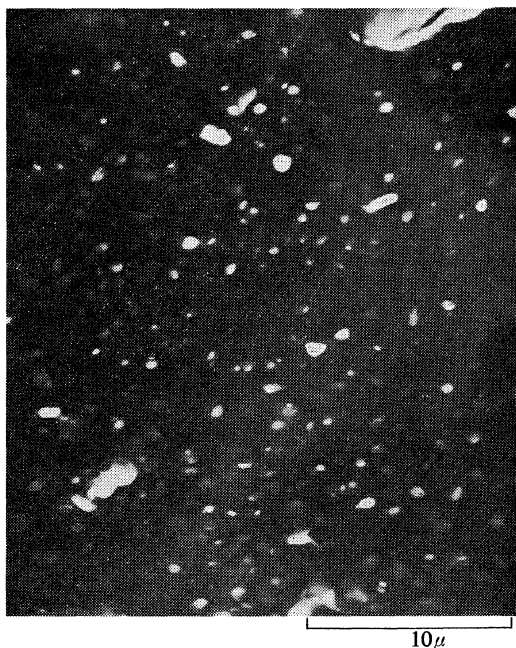
EM #1. Intraparticle pore distribution of solution resin at 2200 \times .
