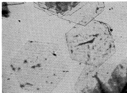
Figure 2. Electron micrograph of single crystal of POM grown from m -cresol at 90°C.
