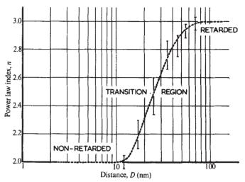
Fig. 1 Variation of power law index, n, of the van der Waals law of force between crossed mica cylinders with distance of separation D. Below 12 nm the forces are non-retarded and the law of force is  $F = AR/6D^n$ , with  $A = (1.35 \pm 0.15) \times 10^{-19}$  J, n = 2, and where R is the radius of the cylinders. Above 50 nm the forces are retarded and the law of force is  $F = 2\pi BR/3D^n$ , with  $B = (0.97 \pm 0.06) \times 10^{-28}$  J m, n = 3.
