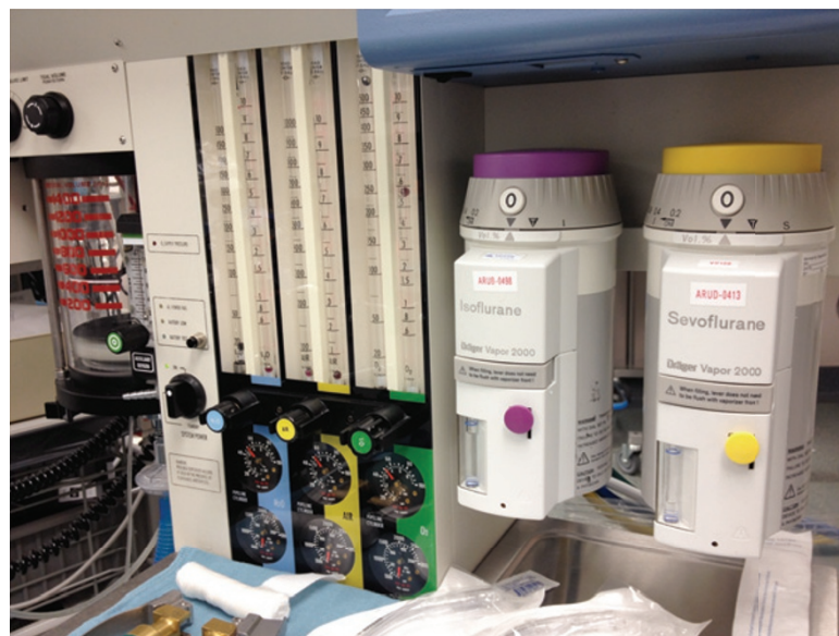
Figure 3 | Anesthesia machines were engineered for safety, with multiple design elements demonstrated in this display. Vapour knobs are large, colour coded, and turn on and off in the same direction across the circuit. The nitrous knob is linked to the oxygen system to prevent hypoxic gas mixtures and disconnect alarms are present and audible.
