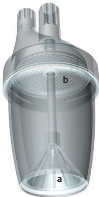
Figure 7 | The disposable FLOTAC fecal sampling kit. This consists of a collector (a) and a filter (b).
