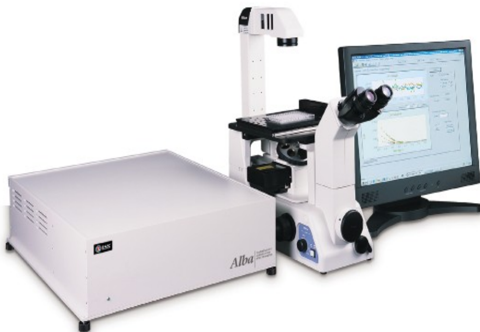
Fig.1.4. The FCS Alba™ Microspectrometer System manufactured by ISS Co., (Urbana, Illinois, USA). The inverted, epi-fluorescence microscope shown in the figure is the Nikon TE-300 –special Model, that has available both a back illumination port and a left-hand side port. The PC employed for data acquisition, storage and processing is located behind the instrument, as is the laser illumination source (not visible in the figure).
