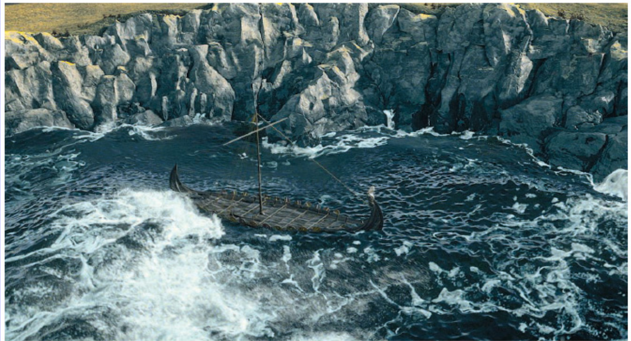
Realistic simulations. A simulated ship upon a simulated ocean. Here, the film industry's Naiad software is used to evolve the incompressible Navier-Stokes equations for the water, strongly coupled with the rigid-body dynamics of the longboat, with additional phenomenological simulation of foam and spray.
