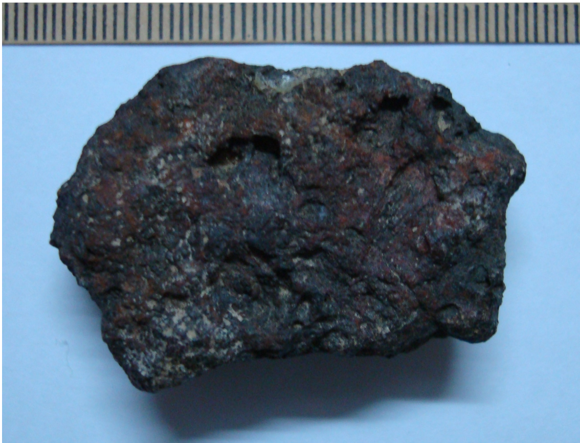
Figure 3. Meteorite debris specimen (scale: mm) tested using XRD and WD-XRF analyses.
