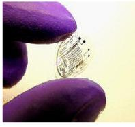
Flexible electronics embedded in contact lens
