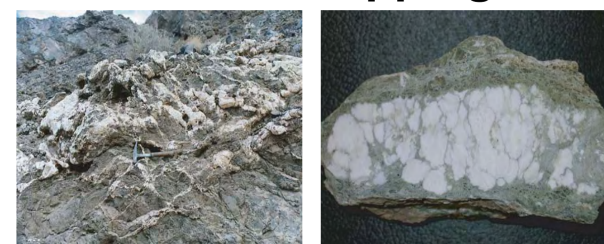
Natural Analog: Magnesite filled fractures in Oman CaAl_2Si_2O_8 + CO_2 + 2H_2O = CaCO_3 + Al_2Si_2O_5(OH)_4 (Matter et al., 2006)
