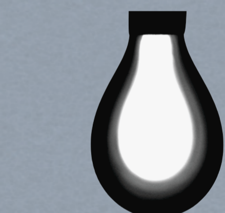
Figure 6: Sample H 2 O drop in liquid CO 2 at 5.44 MPa & 291 K.
