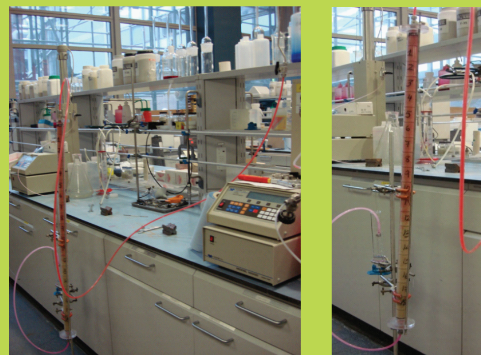
Sand-packed column injected with non-wetting fluid (oil dyed red).
