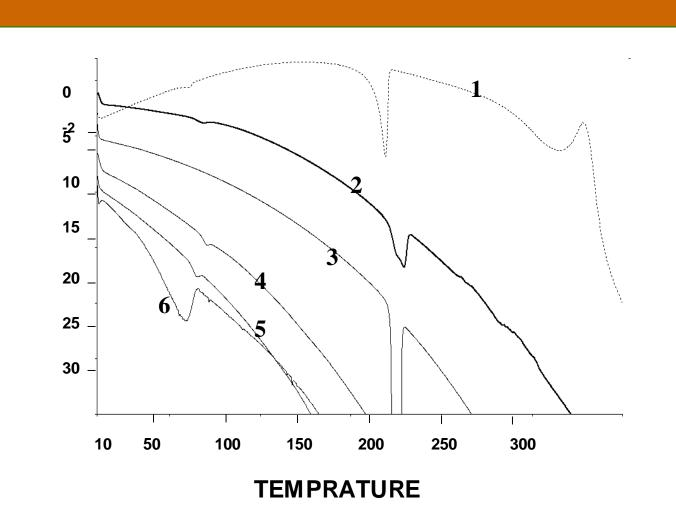
DSC thermograms showing melting temperature of PLA matrix(curve-2) containing Isoniazid( curve-1), Rifabutin(curve-6) and conbination of both (curve-5). Isoniazid(curve-3) and rifabutin (curve-4)
