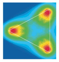
Surface plasmon modes of a silver nanoprism mapped in an electron microscope.
