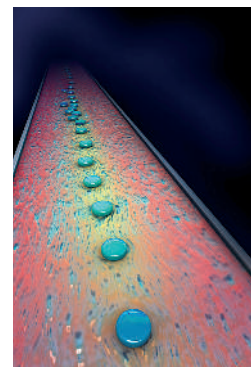
A one-dimensional crystal of water droplets in oil supports slow-moving phonon-like modes.
