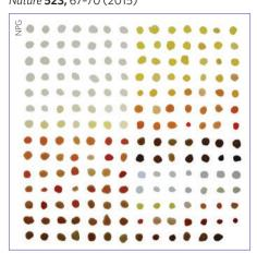
How many scientists would love to have a small and cheap spectrometer? Jie Bao and Moungi Bawendi have come up with a solution by integrating almost two-hundred absorptive filter arrays made of colloidal quantum dots and a charge-coupled device detector into a coin-sized digital camera capable of resolving spectral peaks separated by mere nanometres. Such resolution and compactness may find applications in medicine or space exploration.
