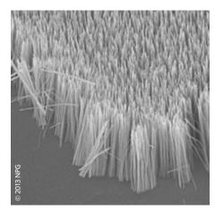
It is not hard to imagine the consequences of setting a field on fire. But what happens when an intense femtosecond laser burns though a micrometre-sized field — an array of nanowires? Michael Purvis and colleagues have done the experiment and found that it's a good way of producing dense, ultra-hot plasmas, rivalling those created in the pursuit of thermonuclear fusion.
