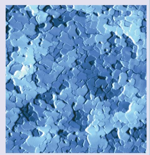
takes place. The surface morphology as captured by atomic force microscopy (pictured) then shows signs of double spiral defects. A hexagonal-ice bilayer twisting around a double screw axis preserves the hexagonal structure. The formation of intertwined double spirals requires more elastic bending than single spirals, but the authors argue that the associated energetic cost is compensated by the higher stability of hexagonal ice.
