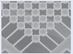
period of the structure and the thickness of the nanoresonators were 1.2  $\mu m$  and 300 nm, respectively.
