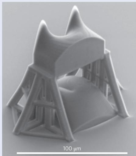
After printing, the structures were rinsed in developer and treated with isopropanol for clean-up. The volumes of the two components (transformer and corrector) are  $60 \times 60 \times 32 \mu\text{m}^3$  and  $60 \times 30 \times 51.5 \mu\text{m}^3$ , respectively; the two components were separated by a distance of  $60 \mu\text{m}$ .
