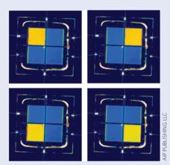
the photonic crystal resonance. The result is a structure that acts as a highly efficient narrowband absorber, or thermal emitter (once hot), of mid-IR light (wavelength of ~9.1  $\mu$ m) with a Q factor of ~70. The device is heated by applying an electrical current that flows through the lower n-GaAs layer.
