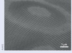
from the object surface. If one knows the local height of the object relative to the flat surface and the direction of propagation and the wavenumber of light in the surrounding medium, it is simple algebra to calculate the local phase variation induced by the object's presence. Then one places resonators whose phase response locally compensates for the variation.
