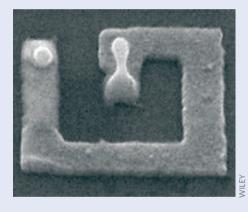
Photonics. "As a consequence, our laser beam starts by melting the nanostructures precisely in the plasmonic hotspots and creates tiny pools of melted gold therein. Within these pools, hydrodynamic processes can take place, such as the nanojets seen in our images."
