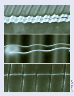
Irradiating the target with 5 ns laser pulses at intensities of 0.07-0.2 GW cm<sup>-2</sup> caused the ablative coating to vapourize into a plasma. The expanding plasma bounced off the confining media to generate a strong shock pressure of 600-1,000 MPa, which was sufficient to shape the metal foil — and thus the underlying NWs — onto the mould.
