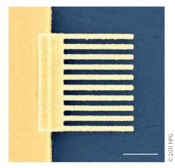
Scientists from the University of Cambridge and the University of Manchester in the UK have shown that introducing gold—titanium plasmonic nanostructures next to the electrical contacts of a graphene photodetector can significantly enhance its maximum voltage. The role of the nanostructures is to covert incident light into plasmonic oscillations and guide electromagnetic energy to the detector's p—n junction. The team experimented with
